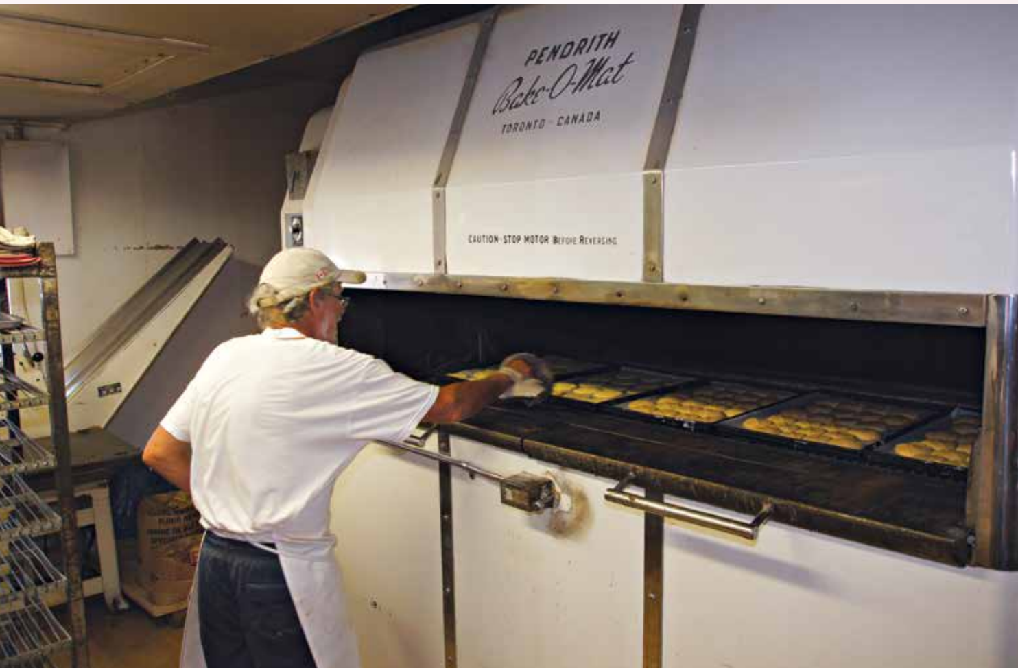
▲ The baking is done. Paul Holman putting his hand into the mouth of the oil-fired Pendrith Bake-O-Mat.
